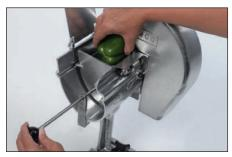
Loading the Easy Slicer is a cinch. Just place your produce in the trough behind the blade, close the cover plate and go.
